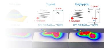
Parameter: I=200 A; TS=4.5 mm/s; WFS=4 m/min; D<sub>L-A</sub>=10 mm; P=5 kW.
