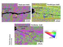
• A K Syed, X Zhang, A E Davis, J R Kennedy, F Martina, J Ding, S Williams, P B Prangnell. Effect of deposition strategies on fatigue crack growth behaviour of wire + arc additive manufactured titanium alloy Ti-6AI-4V. Materials Science & Engineering A (Accepted on 27/03/2021).
