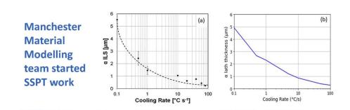
Recently, the Materials Modelling team at University of Manchester have begun to model the beta to alpha solid state transformation (SSPT) in Ti64. They hope that this can be used to complement experimental observations of alpha lath growth in Ti64. This may possibly offer insights into how the addition of extra alloy elements, and the alteration of thermal conditions, affects the lath growth and hence the microstructure.
