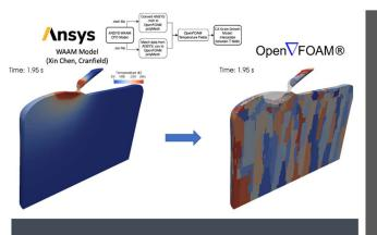
Manchester microstructure modelling team coupled cellular automata grain growth model to Cranfield WAAM CFD model
