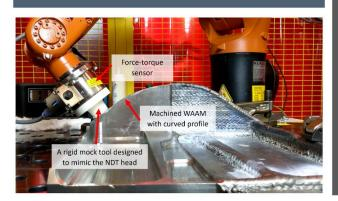
A controller was designed in the LabVIEW platform to update the robot's pose in real-time based on the feedback from the force-torque maintain a constant force between the NDT sensor (UT roller-probe / of the WAAM during the surface of the WAAM during the scan.
